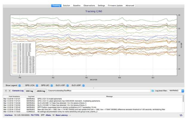
Open *Tracking* tab. Wait until at least 5 satellites have signal strength above 33 dB-Hz and Piksi computes a Single Point Solution or SBAS solution. The POS LED on Piksi Multi will show solid orange once it has a position solution.
