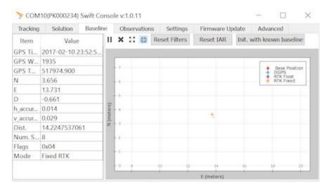
If the surveyed position was programmed on the base station and broadcasting was enabled (see *Configuring Base Station Radio Messages* above) you can see the rover's position on the Solution - RTK Position tab.
